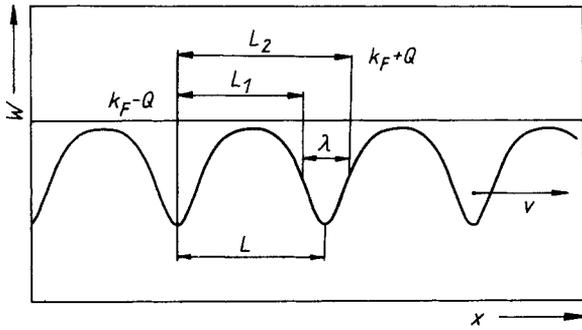
Fig. 1. The deformation field  $W(x)$  with period  $L$  moving with a speed  $v = \hbar Q/2m$ .  $L_1, L_2$  are the periods of the deformation field for quasi-particles with impulses  $k_F - Q$  and  $k_F + Q$ , respectively
