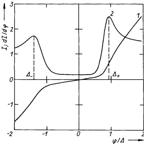
Fig. 3. (1) Current–voltage and (2) conductivity–voltage characteristics of the superconducting current
