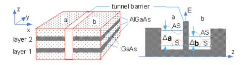
Fig. 1. A pair of two-layer FQHE systems connected by a tunneling barrier.
