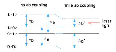
Fig. 2. Change of energy level by the introduction of tunneling coupling between a and b systems.
