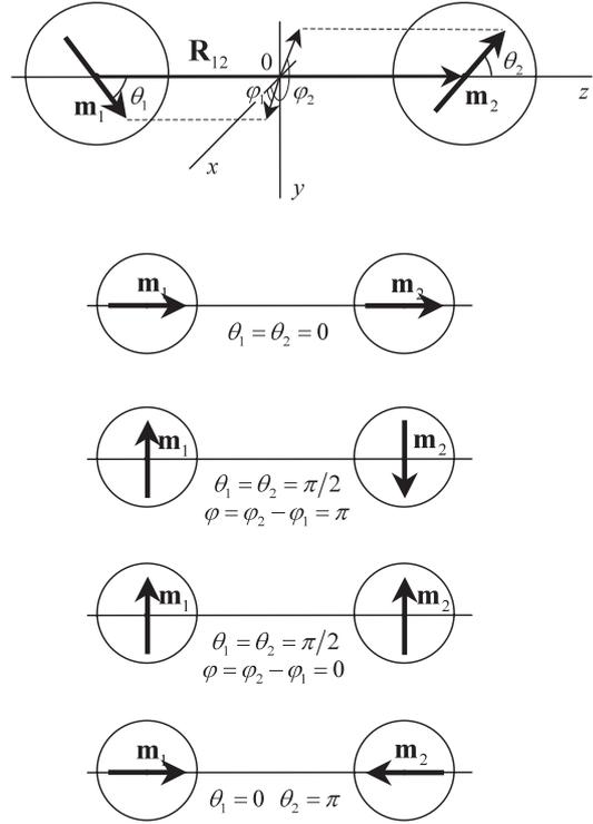
**Figure 2.** The four energy saddle points of a pair of ferromagnetic quantum dots, as defined in equation (20). Of these four, either 1 and 2 is the ground state, depending on condition equation (22). States 3 and 4 are never stable.
